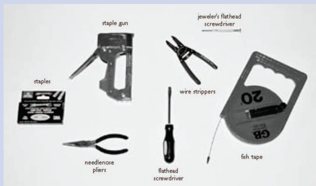
Figure 3. Tools to use in installing a loop system. (This and Figures 4-6 are from the Field Quick Start Installation Guide , published by Phonic Ear.)
