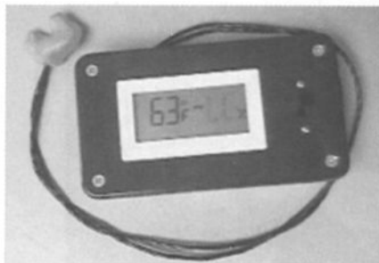
Fig. 1. The test hearing aid connected to the temperature and relative humidity measuring device.
